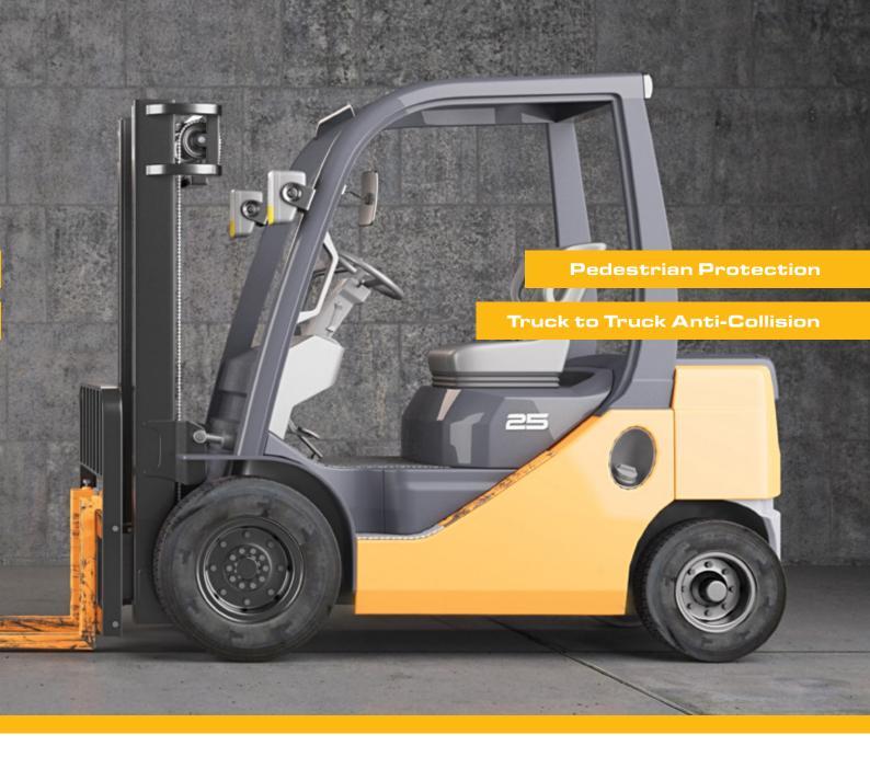
zones such as doorways or blind corners RFID tags are installed, when the vehicle enters the area the truck based unit detects the tag and activates a speed limiter on the vehicle, the zones can be as small or as large as required.
